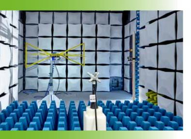
You as our customer will gain from our modern test equipment. With the help of our FAR chamber the time-consuming height scan that is required by standards for partial absorber rooms is obsolete. In addition, our fast FFT-based emission measurement ensures that a peak value measurement over a complete frequency band is already completed after a very short time.
